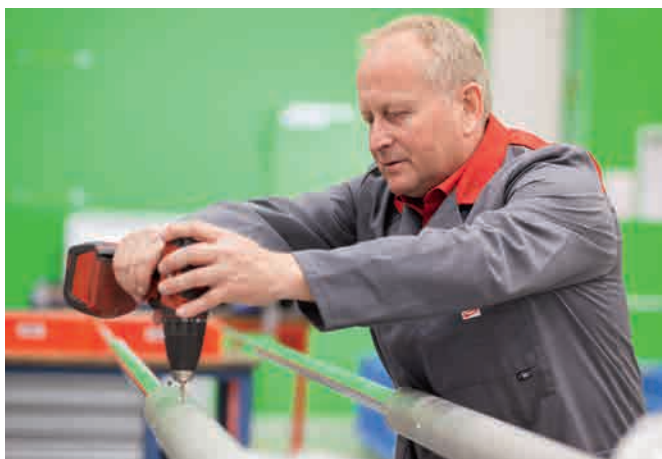
Air-termination rods with special lengths
